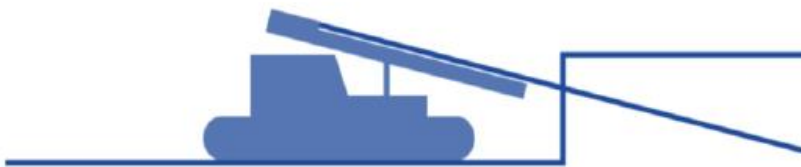
2 Drilling nail hole
