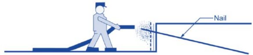
4 Application of sprayed concrete facing
