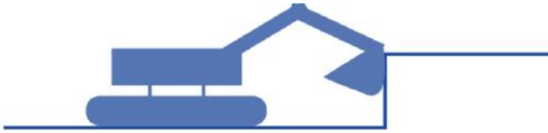
1 Excavation of appropriate lift height
