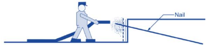
4 Application of sprayed concrete facing
