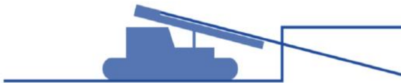
2 Drilling nail hole
