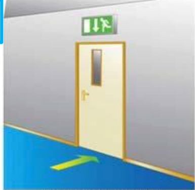
at each exit door intended to be used in an emergency
